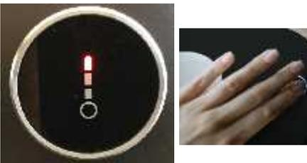
On the temperature dial, select 1 to proceed with descaling or select 0 to cancel, then press and release the brew button. The Ristretto button will blink throughout the entire process.
