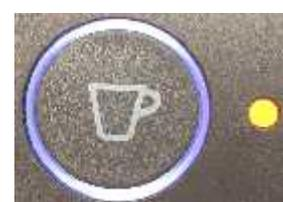
If the maintenance light is on when the machine is turned back on, this is normal. Run a Lungo cycle without a capsule and the light will go out as soon as water begins to flow into the machine.
