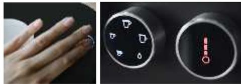
With machine off and slider closed, press and hold the brew button until both dials flash 3 times.
